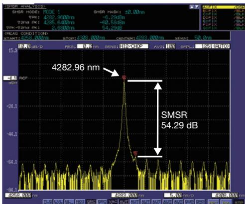
Measurement example of 4.3  $\mu\text{m}$  DFB laser
